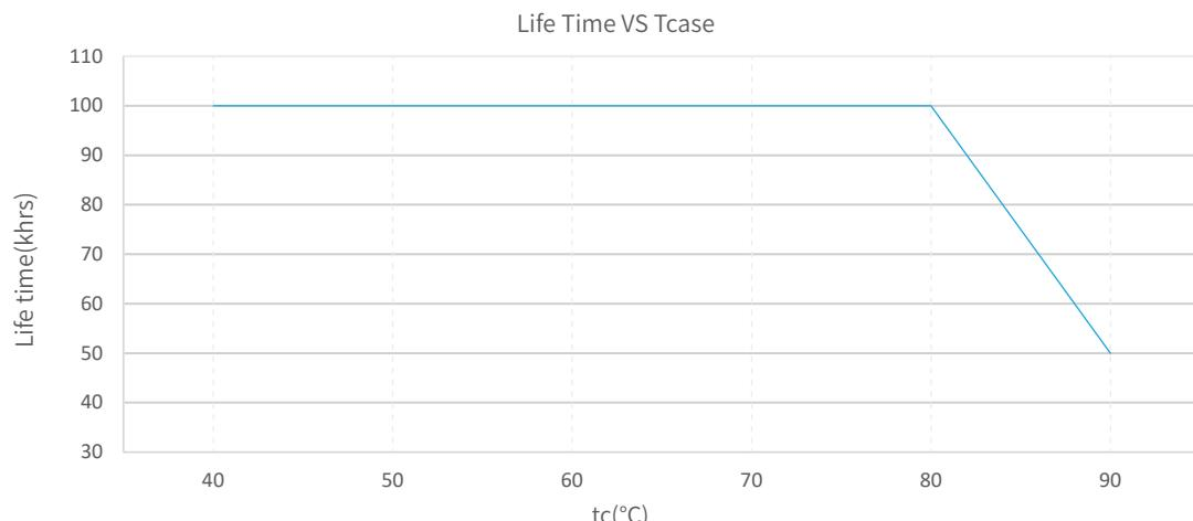
The life-time of the LED driver is shown in the figure above calculated (based on the 90% survival rate). The relation of tc to ta temperature depends also on the luminaire design.
