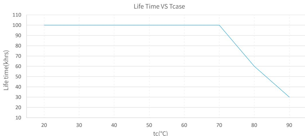
The life-time of the LED driver is shown in the figure above calculated (based on the 90% survival rate). The relation of tc to ta temperature depends also on the luminaire design.
